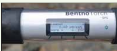
A Benthos-Torch, new technology to measure algae, cyanobacteria and diatoms.
