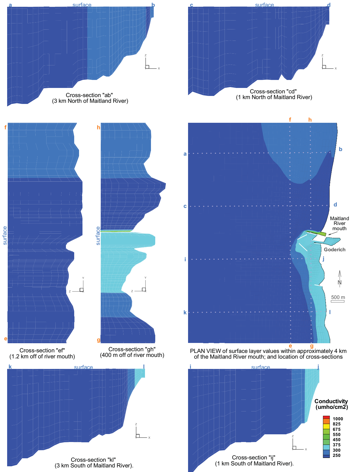
Figure 5.4C(b) Conductivity, (plan view and 6 cross-sections), at 00 hours on November 14, 2003. [Note: the depth ("z"-dimension) is exaggerated 300 times].
