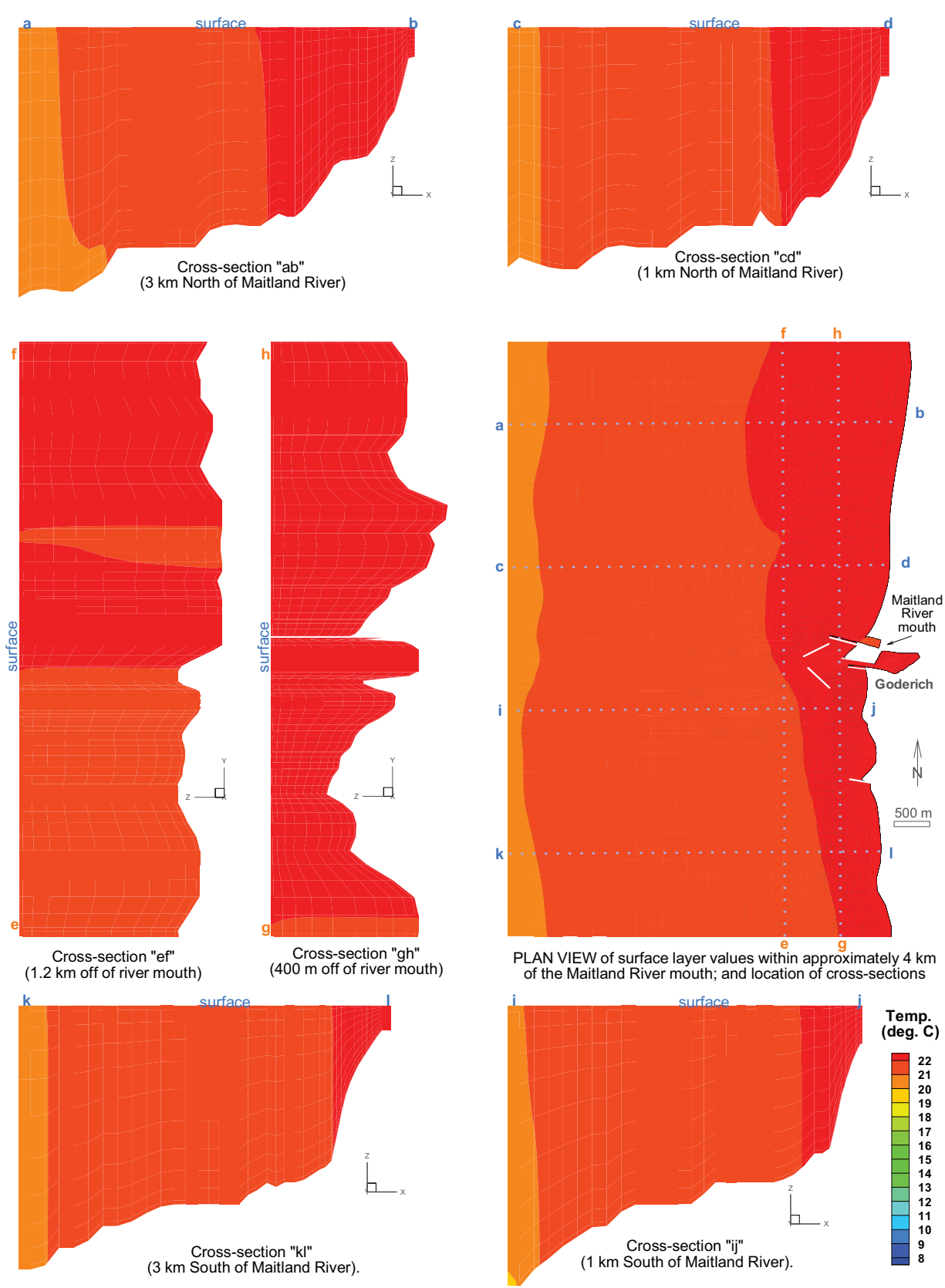
Figure 5.2T(b) Water temperature, (plan view and 6 cross-sections), at 00 hours on July 21, 2003. [Note: the depth ("z"-dimension) is exaggerated 300 times].
