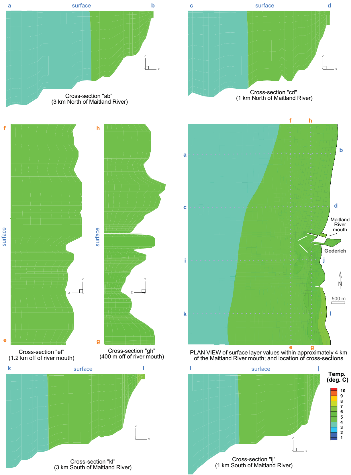
Figure 5.1T(j) Water temperature, (plan view and 6 cross-sections), at 00 hours on April 4, 2003. [Note: the depth ("z"-dimension) is exaggerated 300 times].
